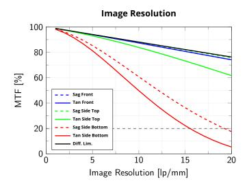
Modulation Transfer Function (MTF) vs. Image Resolution, wavelength range 486 nm - 656 nm of cylindrical object of diameter 20 mm and height of 15 mm, at wf/N=16
